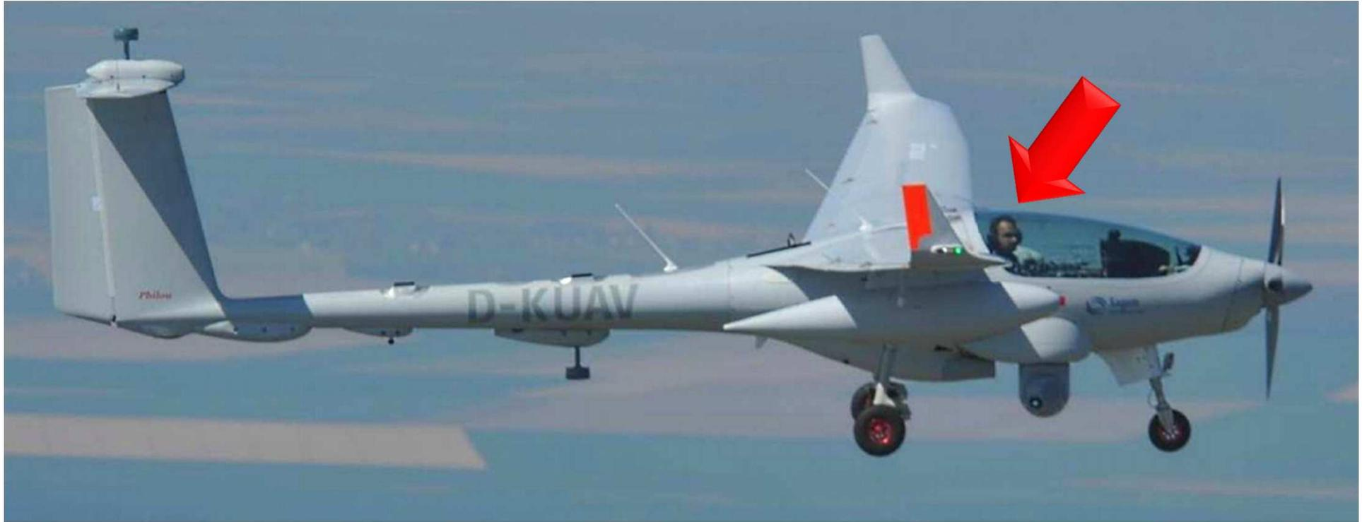
*Take-over by pilot possible during any flight phase using emergency push button*
