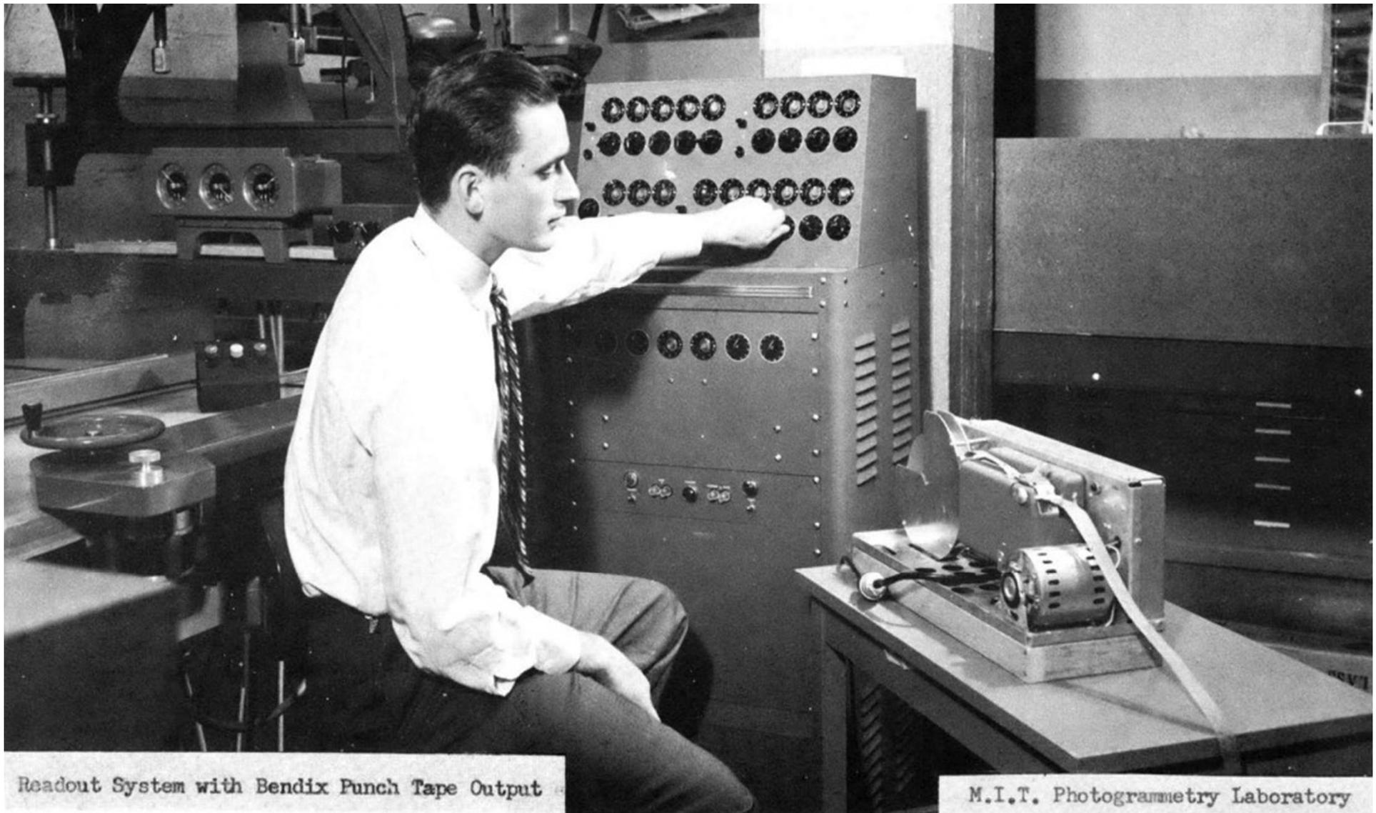
Readout System with Bendix Punch Tape Output
